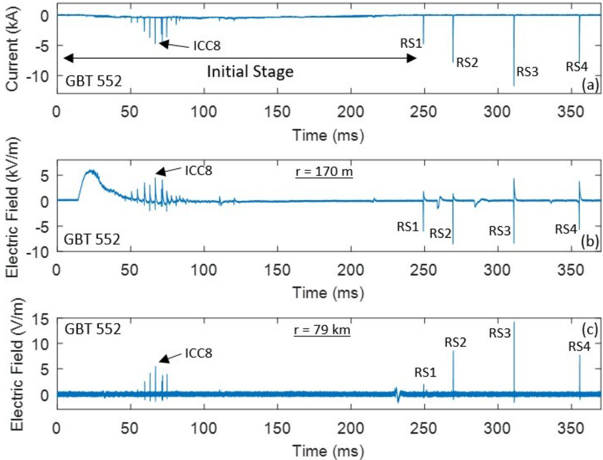
Fig. 1. (a) Current, (b) electric field at 170 m, and (c) electric field at 79 km for the upward negative flash GBT #552, shown on a 400-ms timescale. The initial stage was followed by four downward leader-return stroke sequences. An expanded version of one of the ICC pulses (ICC8) occurring during the initial stage of this flash is shown in Figure 2.
