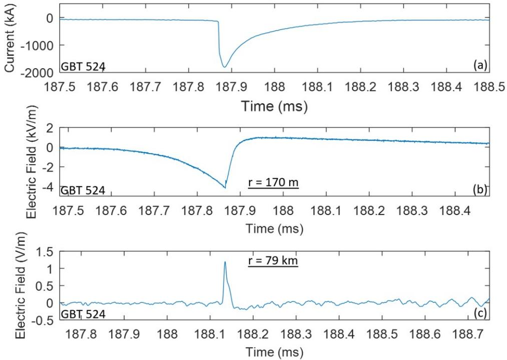
Fig. 4. (a) Current, (b) electric field at 170 m, and (c) electric field at 79 km for a negative unipolar ICC pulse overlaid on negative IS background current in upward negative flash GBT #524, shown on a 1.0-ms timescale.
