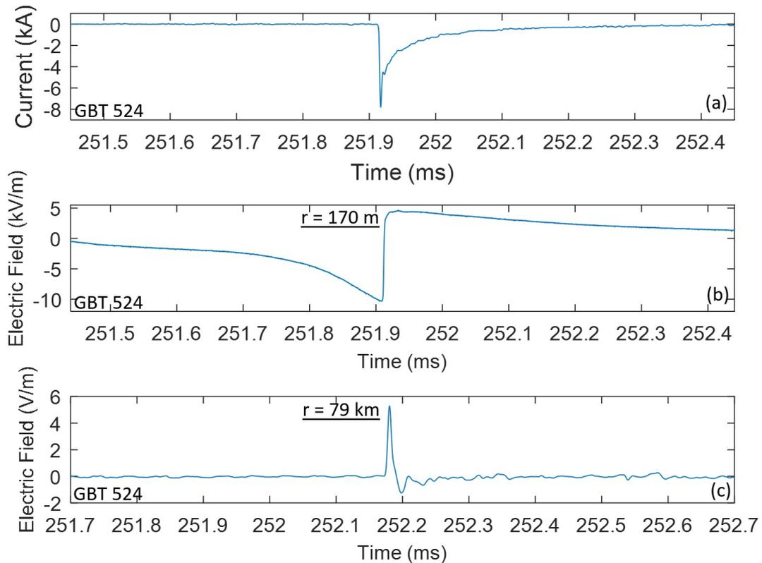
Fig. 5. (a) Current, (b) electric field at 170 m, and (c) electric field at 79 km for a negative return stroke in upward negative flash GBT #524, shown on a 1.0-ms timescale.
