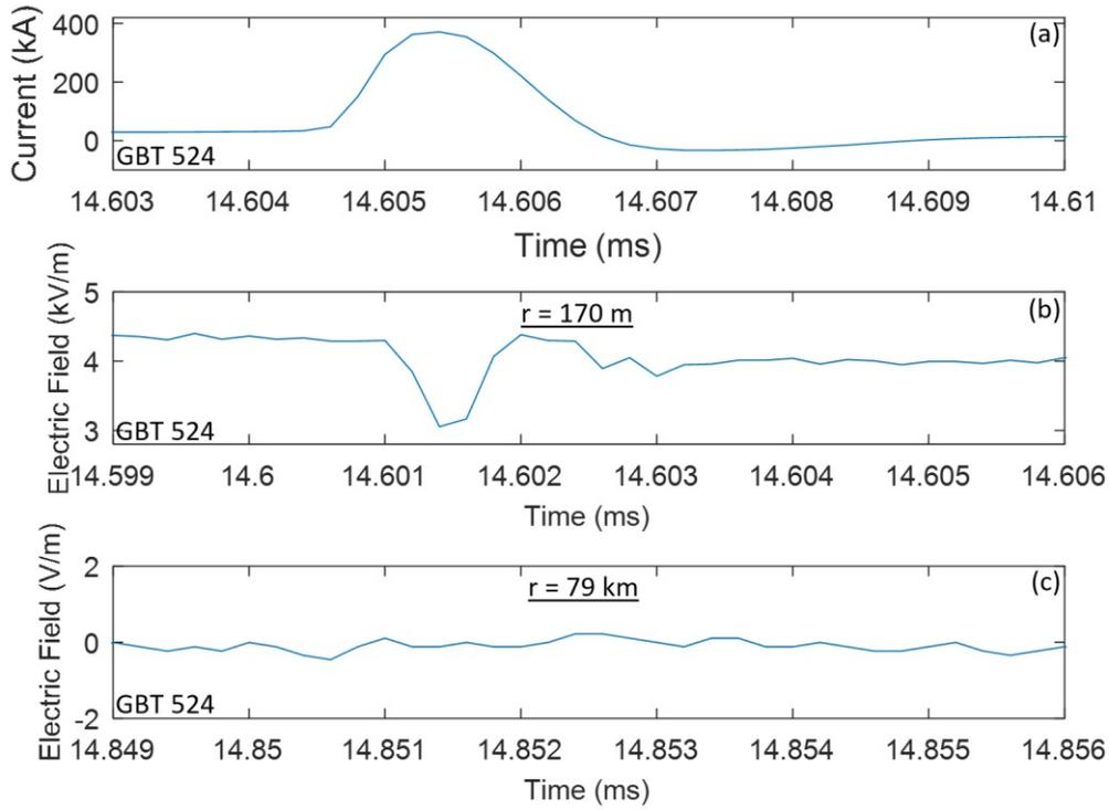
Fig. 3. (a) Current, (b) electric field at 170 m, and (c) electric field at 79 km for a positive bipolar ICC pulse overlaid on positive IS background current in upward negative flash GBT #524, shown on a 7- $\mu$ s timescale. The signal-to-noise ratio of the corresponding radiation field signature at 79 km was not sufficient for it to be measured as seen from (c).
