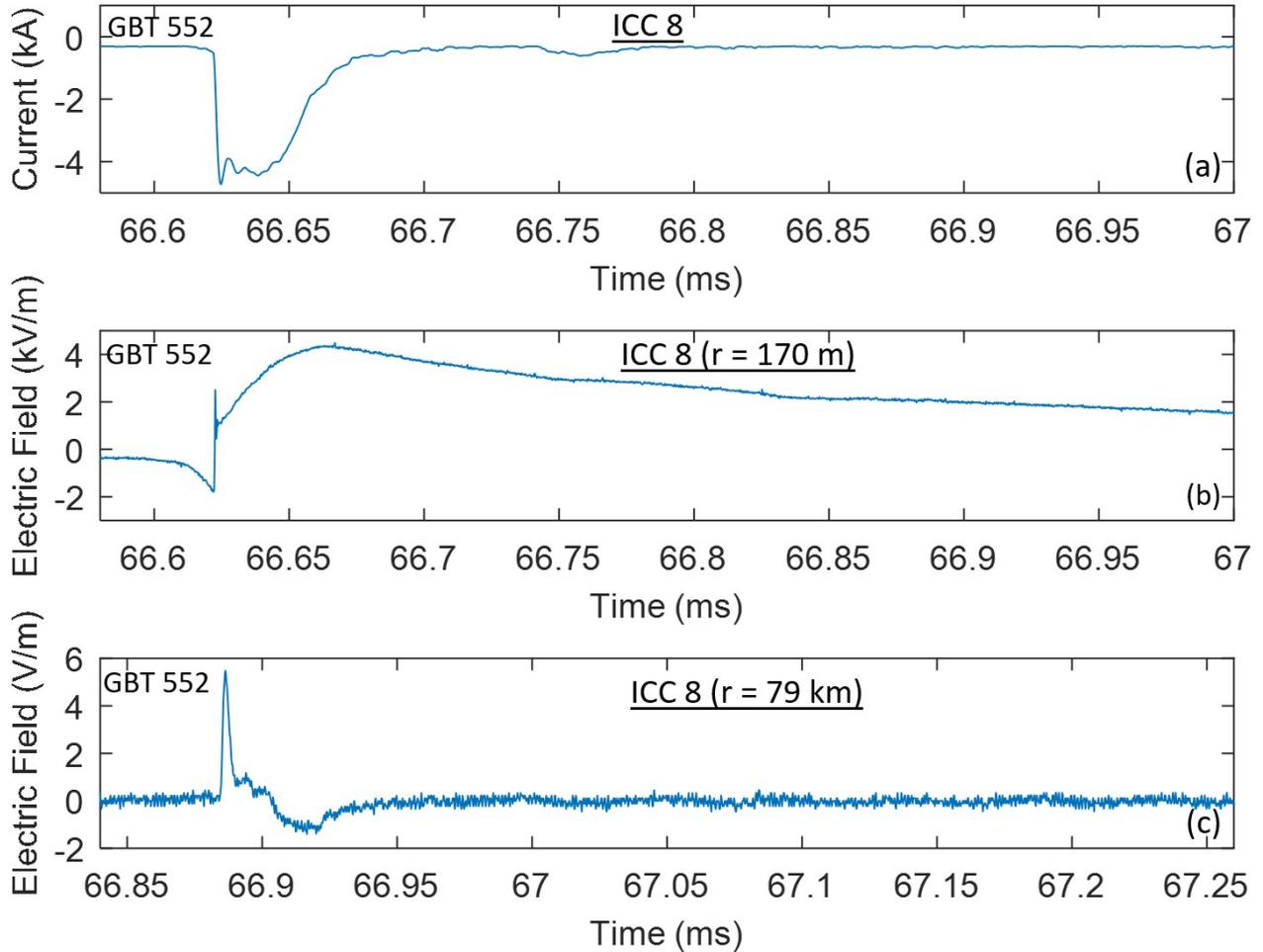
Fig. 2. (a) Current, (b) electric field at 170 m, and (c) electric field at 79 km for ICC8 in upward negative flash GBT #552, shown on a 420- $\mu$ s timescale. See Figure 1 for more details.
