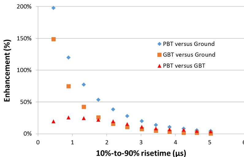
The simulation results in Fig. 5 support the observation of LLS overestimation of the stroke peak currents, as for the same lightning stroke to the two towers the LLS sensors will see slightly higher peak fields in case of the PBT.
