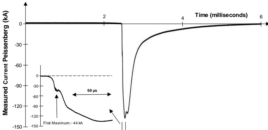
Fig. 7: Current of a negative first stroke measured at the PBT on July, 03, 2015 (#365).
