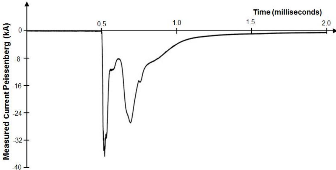
Fig. 6: Current of a negative first stroke measured at the PBT on August, 22, 2011 (#331).
