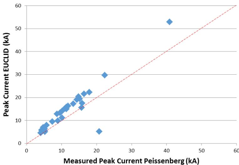
Fig. 4: Measured peak currents at the PBT versus BLIDS/EUCLID peak currents for subsequent strokes. Dashed red line (slope=1) is the locus of points for which the BLIDS/EUCLID peak currents and Peissenberg peak currents are equal.
