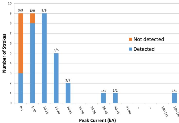
Fig. 2: Number of detected strokes versus peak current. For each peak current range (bin size of 5 kA), the ratio given on top of the column indicates the number of strokes detected by the BLIDS/EUCLID (numerator) and the number of strokes recorded at the Peissenberg (denominator), for that peak current range.
