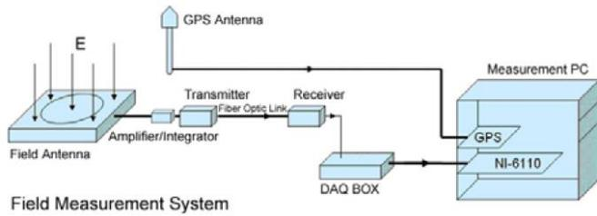
Fig. 4. Schematic representation of the system to measure the transient electric fields of lightning discharges [10]
