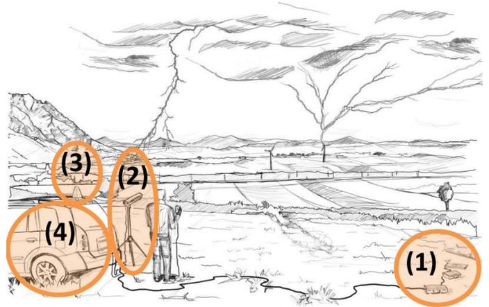
Fig. 3. Schematic setup of the VFRS operated in the field: (1) Electric field sensor, (2) Camera, (3) GPS antenna, (4) Car with inside components (e.g. data acquisition)
