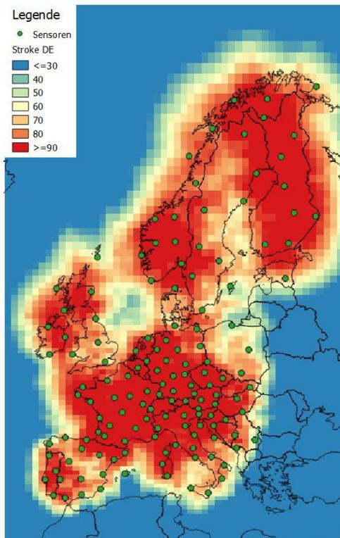
Fig. 7. Modeled stroke DE of the EUCLID network
