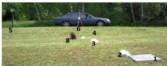
Figure 2: VFRS deployed in the field. 1-flat plate antenna, 2-integrator amplifier, 3-fibre optic transmitter, 4-fibre optic cable, 5-high speed camera, 6-GPS antenna, 7-VFRS components inside the car, 8-power supply. Note: The generator is typically 50 m distant from the car and the antenna deployed.
