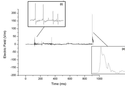
Figure 3: Electric field variations produced during the preliminary breakdown (Region I) and the return stroke (Region II).
