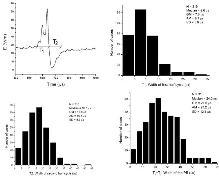
Figure 7: (a) Typical preliminary breakdown pulse (b) T1: width of initial half cycle of pulses (c) T2: width of second half cycle of pulses (d) T1+T2 width of pulses
