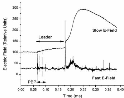
Figure 1: waveform example from electric field changes of the sensors: fast e-field - short decay time and slow e-field – long decay time
