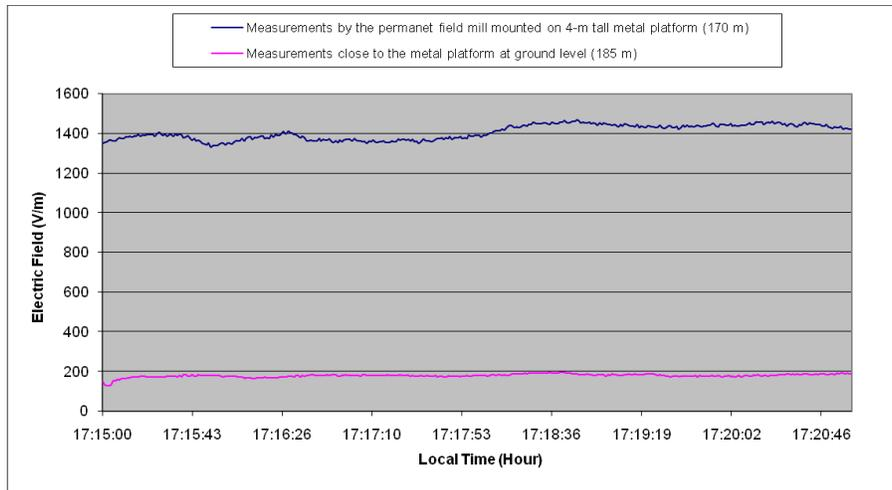
Figure 2: Simultaneously measured fields at the 4-m tall metal platform and at ground level.
