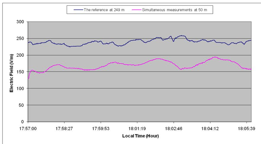
Figure 5: Simultaneously measured fields at distances of 249 m and 50 m from the GBT.
