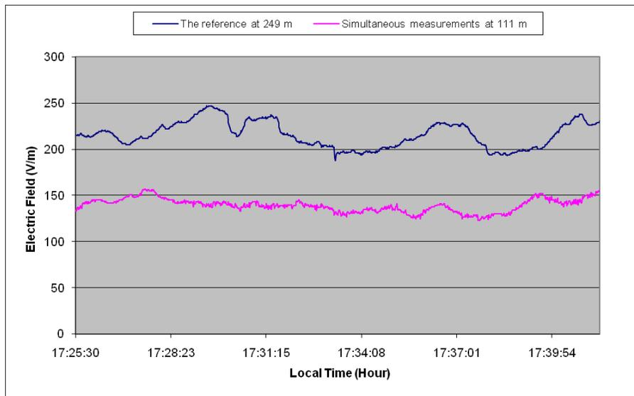
Figure 3: Simultaneously measured fields at distances of 249 m and 111 m from the GBT.
