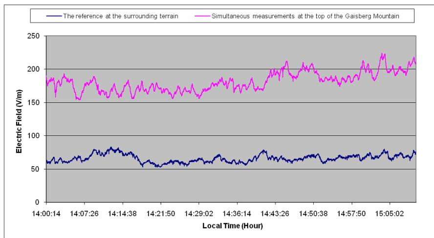
Figure 1: Simultaneously measured fields at the surrounding terrain and at the top of Gaisberg Mountain.
