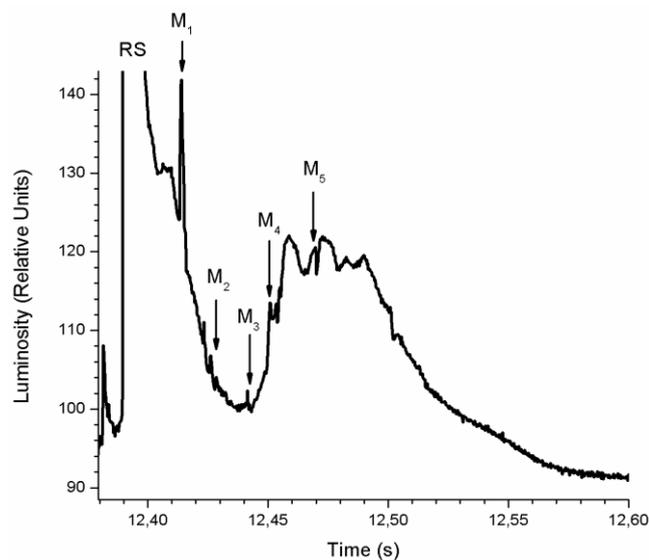
Fig. 2. Luminosity-versus-time curve showing the continuing current period of the selected +CG event. RS indicates the return stroke (which saturated) and M<sub>1</sub> through M<sub>5</sub> identifies the M components analyzed. The luminosity peak that occurs prior to the return stroke was produced by the positive leader.
