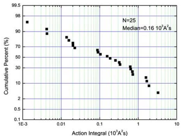
Fig. 5. Cumulative frequency distribution of action integral for upward positive flashes. The sample sizes (N) and median value (Median) are indicated in the figure.
