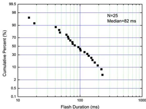
Fig. 3. Cumulative frequency distribution of flash duration for upward positive flashes. The sample sizes (N) and median value (Median) are indicated in the figure.
