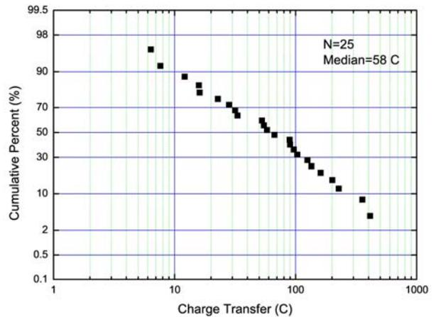
Fig. 4. Cumulative frequency distribution of charge transfer for upward positive flashes. The sample sizes (N) and median value (Median) are indicated in the figure.
