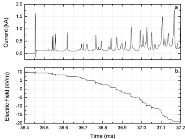
Fig. 6. Simultaneous current and electric field waveforms measured at a distance of 170 m from the GBT for the flash GBT #482, illustrating the high repetition characteristics of current pulses at the initial portion of initial stage current of the upward positive flash.
