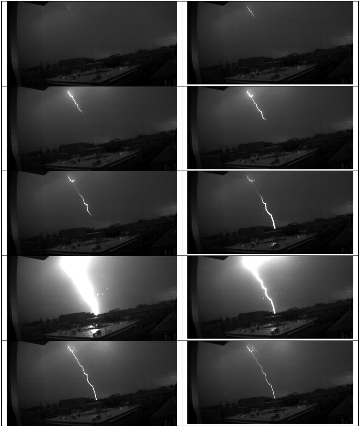
Figure 1- Sequence of frames recorded at 4000 fps of an M component.
