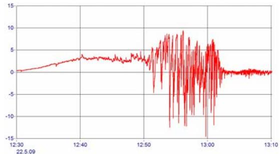
Fig.7: Electric field mill record for the period of lightning activity shown in Fig.6. Field mill is located at a distance of about 170 m from the GBT
