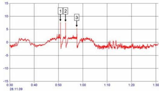
Fig.5: Electric field mill record for 60 minutes period, when lightning activity shown in Fig.4 occurred. Field mill is located at a distance of about 170 m from the GBT. Three lightning events are marked by arrows.
