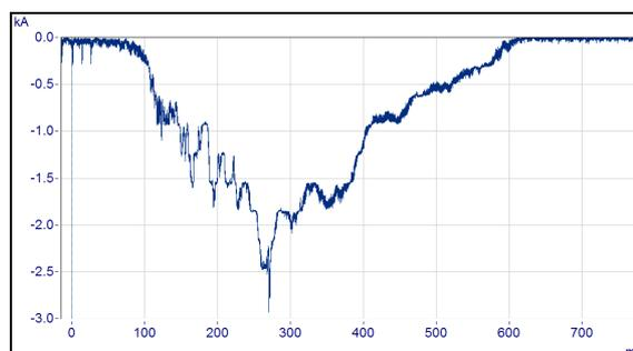
Figure 1 – Current record of flash # 614 with a transferred charge of 546 As
