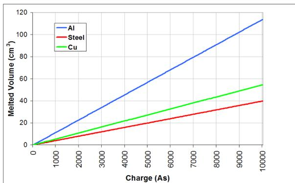
Figure 5 – Estimated melted volume as a function of charge using Eq.(1) for material Al, Steel, and Cu assuming  $u_{a,c} = 30V$ ,  $\theta_u = 20^\circ$
