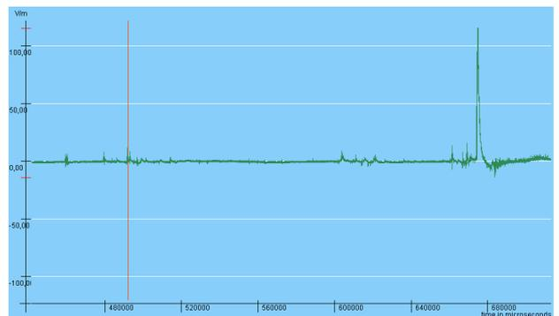
Fig. 4.2: flash #4 with misclassified stroke (vertical red line) 182ms before the +CG stroke.
