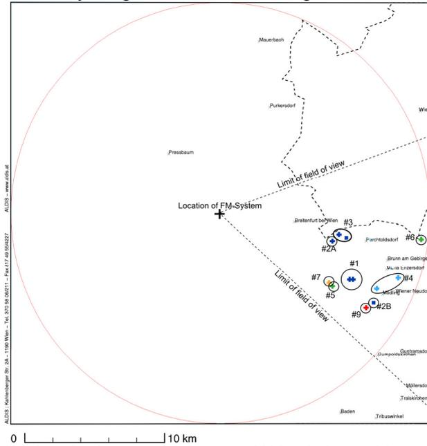
Fig. 3.1: Strokes measured on 1.6.2008 16:12 to 16:31 and categorized as CG stroke by the LLS
