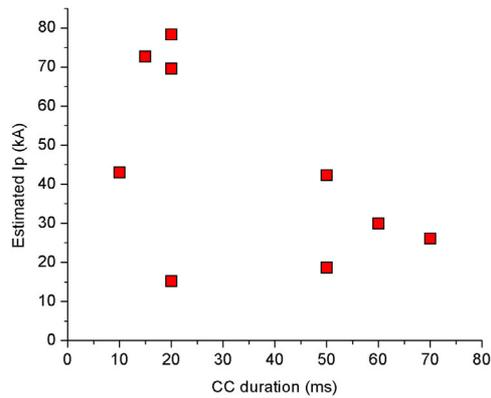
Fig. 4.3: Peak current ( $I_p$ ) versus CC duration for 9 +CG strokes.
