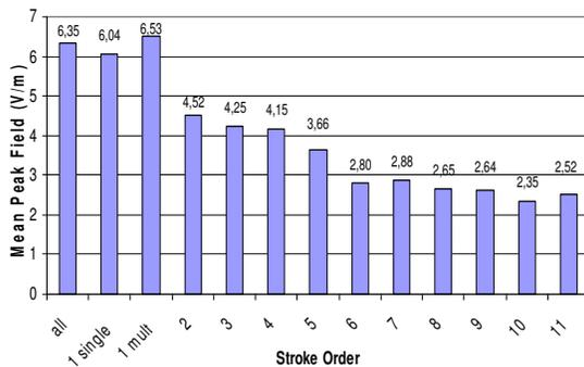
Fig.4.2: Mean peak value normalized to 100 km in V/m versus stroke order of CG strokes of FM data
