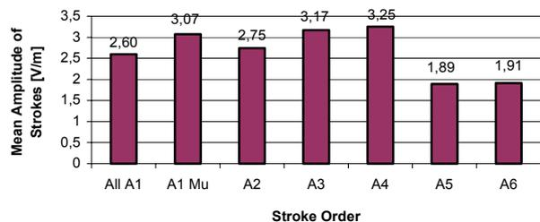
Fig. 4.2: Mean peak value normalized to 100 km in V/m versus stroke order of CG strokes of FM data
