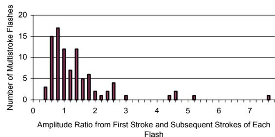
Fig. 4.3: Frequency distribution of the amplitude ratios from all first and their subsequent strokes of multistroke flashes of FM data.
