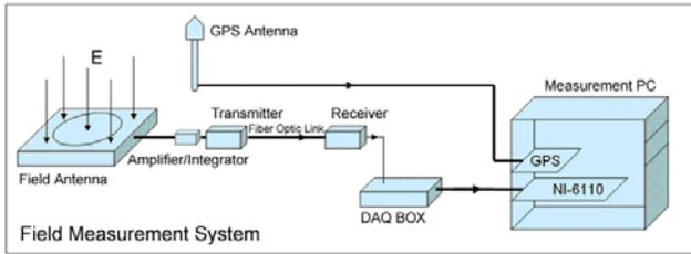
Fig. 2.1: Field measurement (FM) system
