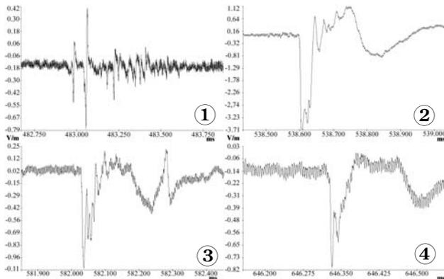
Fig. 3.2: The electric field of a typical negative CG flash (30.08.2004 13:11:53).
