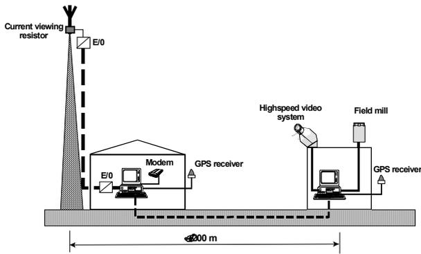
Fig.1: Schematic overview of the experimental setup at Gaisberg tower (E/O: Electrical/Optical signal converter)
