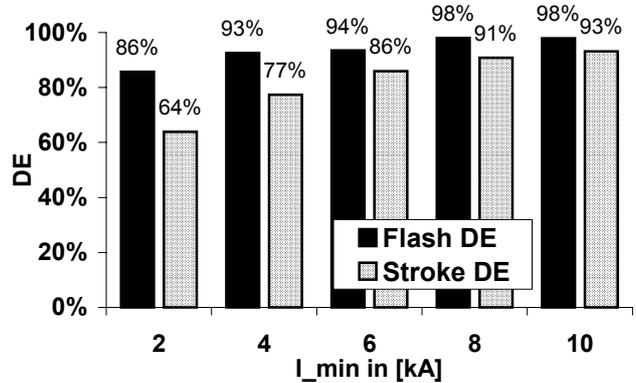
Fig.5: ALDIS flash and stroke detection efficiency as a function of minimum peak current
