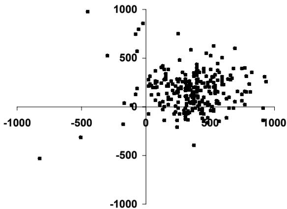
Fig.6: Plot of ALDIS locations for correlated strokes - the tower is located in the origin
