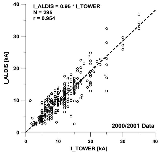
Fig.8: Comparison of directly measured currents  $I_{TOWER}$  with the current estimates from ALDIS
