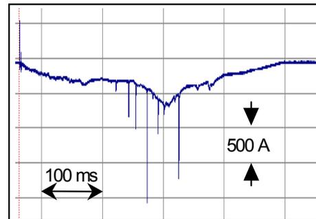
Fig. 4a: ICC-current with 5 ICC pulses flash #182
