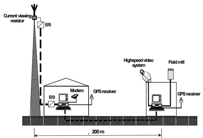
Fig.2: Schematic overview of the experimental measuring setup at Gaisberg tower (E/O: Electrical/Optical signal converter).
