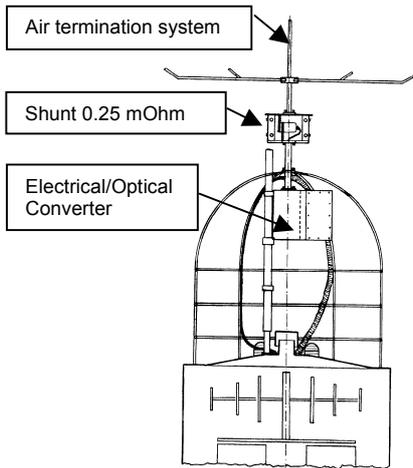
Fig.3: Installed equipment on the tower top
