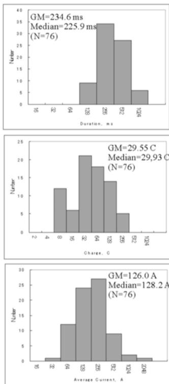
Fig. 3 Initial Stage of object-initiated lightning (Gaisberg, Austria)
