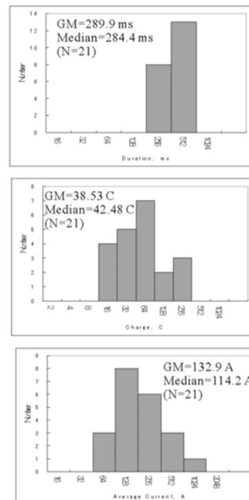
Fig. 2 Initial Stage of object-initiated lightning (Peissenberg, Germany)
