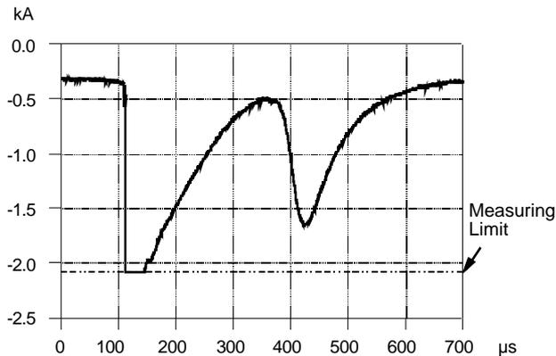
**Figure 7.** Stroke #35 with a double peak current waveshape
