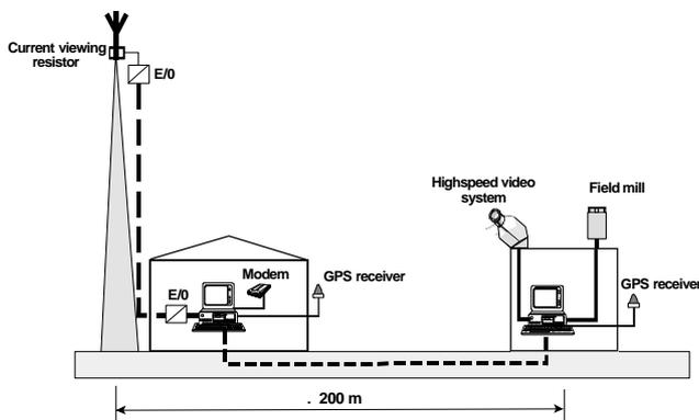
**Figure 3.** Schematic overview of the experimental setup at Gaisberg tower (E/O: Electrical/Optical signal converter).
