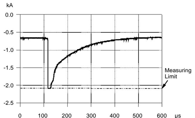
**Figure 6.** Stroke #31 with a "typical" stroke current waveshape
