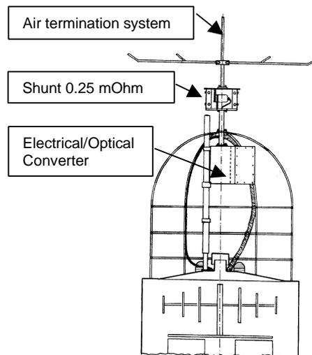
**Figure 4.** Configuration of the measuring equipment on top of the transmission tower
