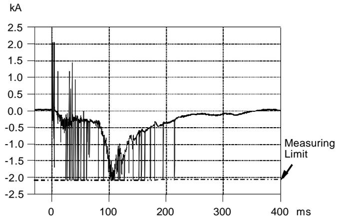
**Figure 5.** Recorded lightning flash current to the Gaisberg tower
