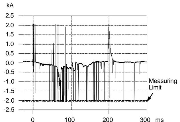
**Figure 8.** Continuing current with bipolar structure superimposed by 39 strokes
