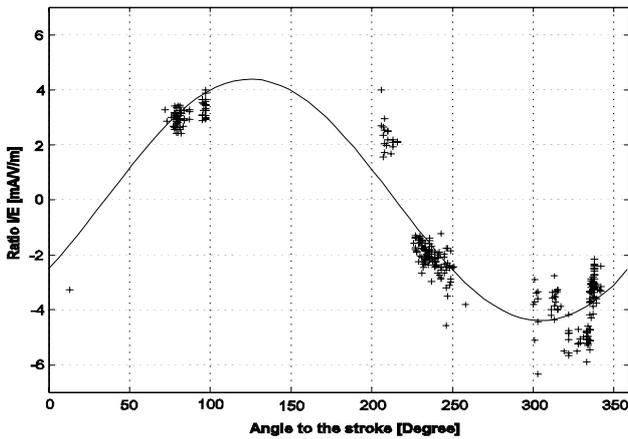
Fig. 3.3: Ratio between peak field and peak current in the cable shield as a function of angle to the lightning stroke
