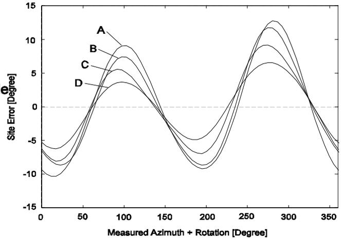
Fig. 2.6: Site error functions for the different grounding conditions of the cable shields
