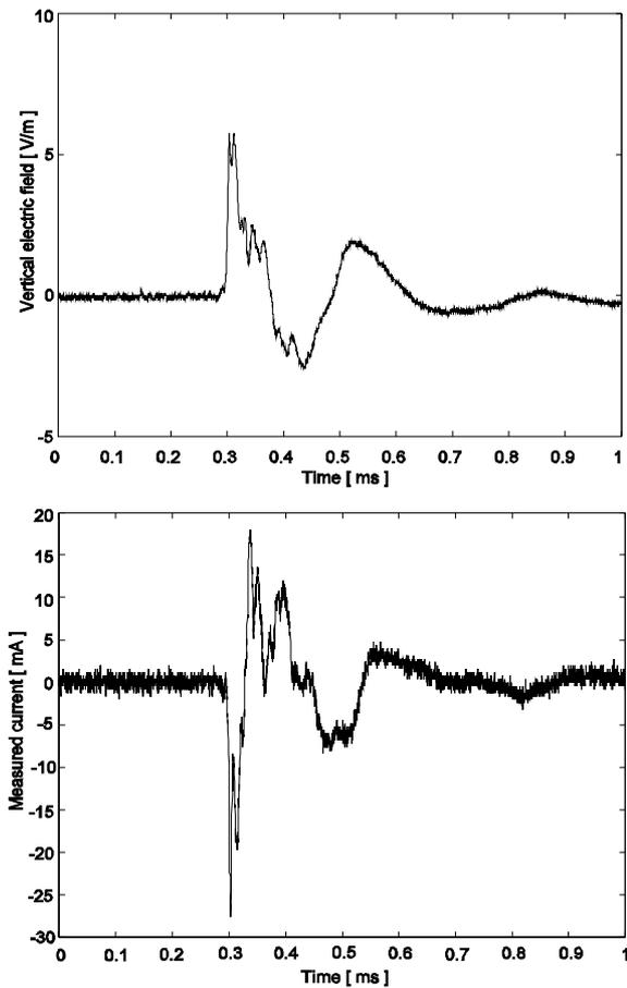
Fig. 3.2: Vertical electric field and induced current in the shield wire of the communication cable of a stroke (04.09.1997 13:38:07.375 UTC)
