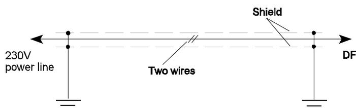
Fig. 2.2: Grounding conditions of the power cable
