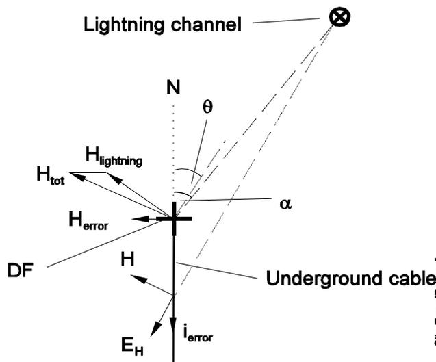
Fig. 2.5: Site error introduced due to an underground cable
